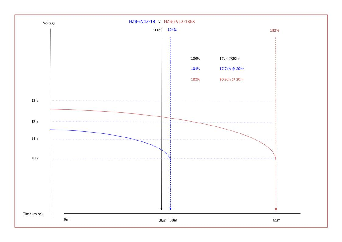
This is a replica of a first cycle comparison capacity test on HZB-EV12-18 and HZB-EV12-18EX.(original test result available on request).
